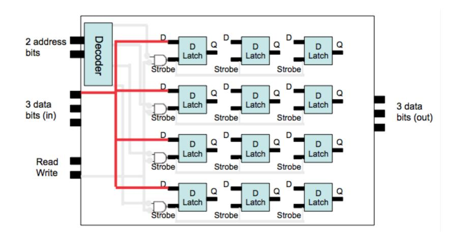
Wire data bits to corresponding memory bits
