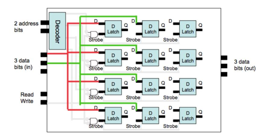
Wire data bits to corresponding memory bits
