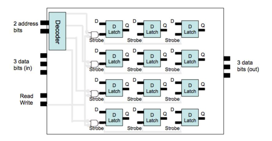
Wire data bits to corresponding memory bits
